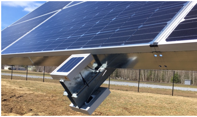
Fig. 3. EETS reference cells mounted back-to-back to capture plane-of-array irradiance measurements for the front and back sides of the tracker. The cells were cleaned twice-weekly.
