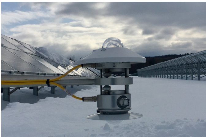
Fig. 15. Albedometer at the Vermont test site. The instrument has two horizontal irradiance sensors, one facing up; the other facing down. The bottom sensor is 1.2 m above the ground.
